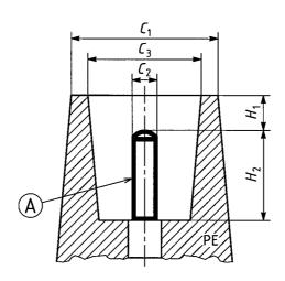
outside diameter of the terminal diameter of the active part of the terminal internal diameter of the terminal distance between the upper part of the
